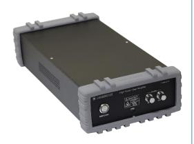
The PMLS provide 1950nm PM Laser light with high stability in both output power and polarization extinction ratio. These advantageously features are intrinsically achieved by using a randomly polarized fiber laser with a specially made high polarization extinction ratio polarizer. The spectral width can be selected as broadband, and 5nm. The power control has several options: fixed and remotely via RS232/USB.
